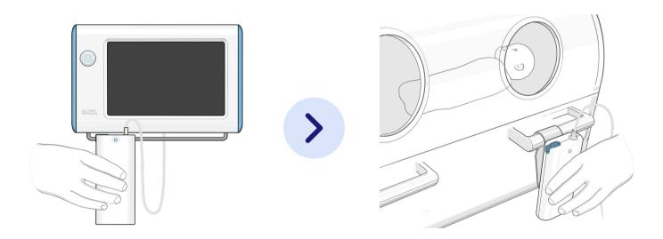
MARNING: Do not position the scanner unit inside a closed incubator or in the infant warming area of a radiant warmer. Doing so may overheat the scanner unit, making the examination end abruptly
